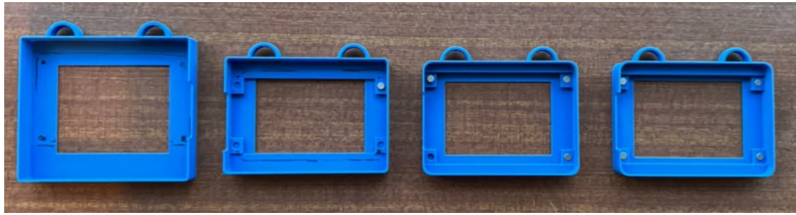
Figure 51 - The four iterations of the box part of the case
