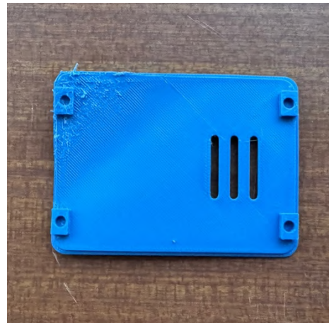
Figure 50 - Printing error of the lid
