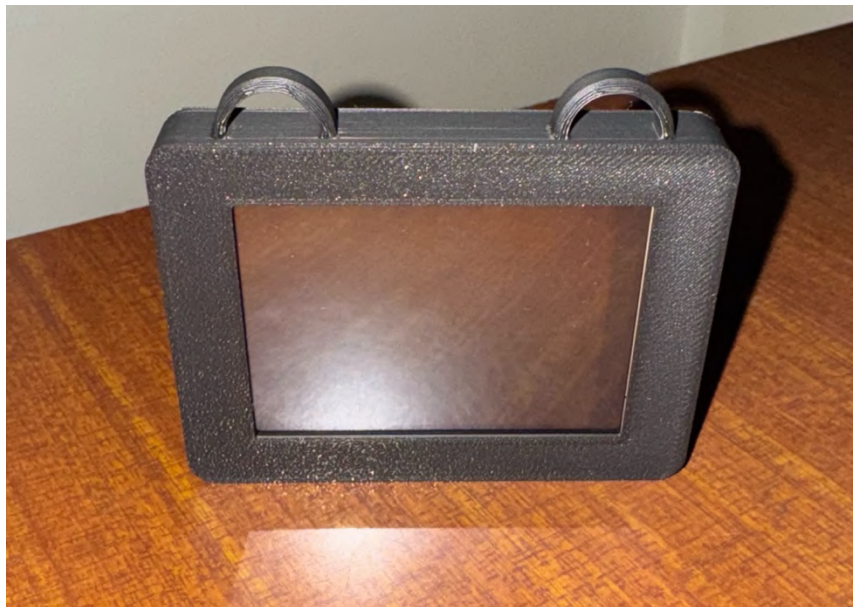
Figure 64 - Photo of the final print of the case assembled with the ESP32 and touchscreen
