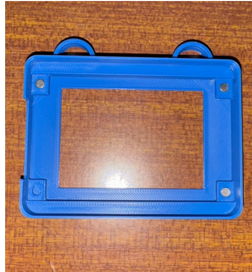
Figure 47 - Third print with magnets
