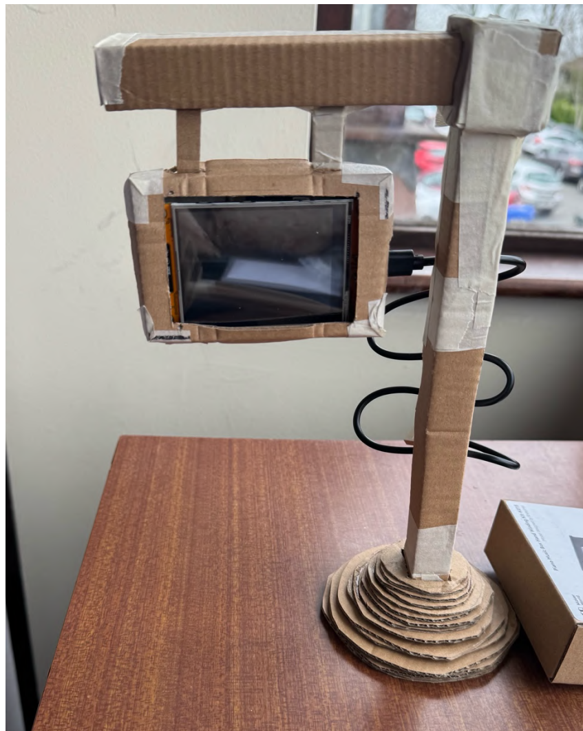
Figure 18 - Full cardboard prototype with ESP32 and touchscreen device
