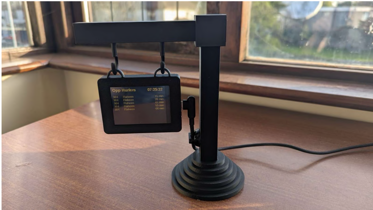
Figure 71 - Prototype assembled with ESP32 and touchscreen turned on and connected to the API
