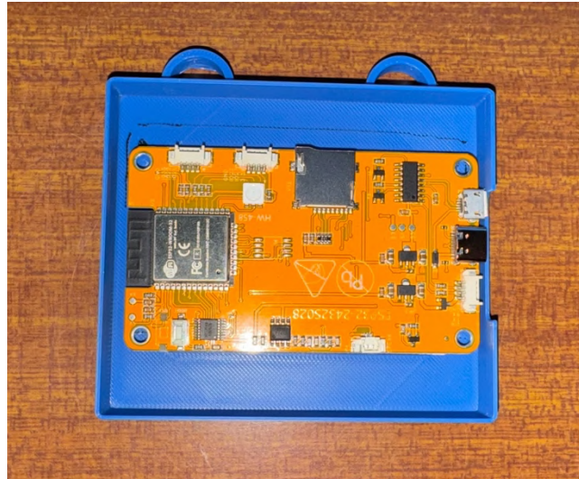
Figure 42 - First print of the case with the ESP32 and touchscreen
