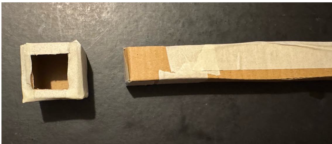
Figure 13 - Vertical pole and connecting cube of the second cardboard prototype
